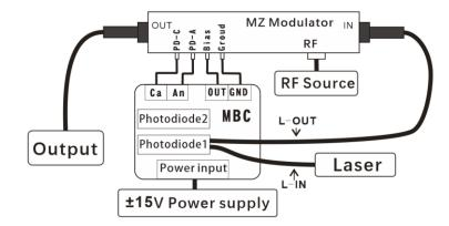
Figure 2. System diagram with controller's on-board photodiode
